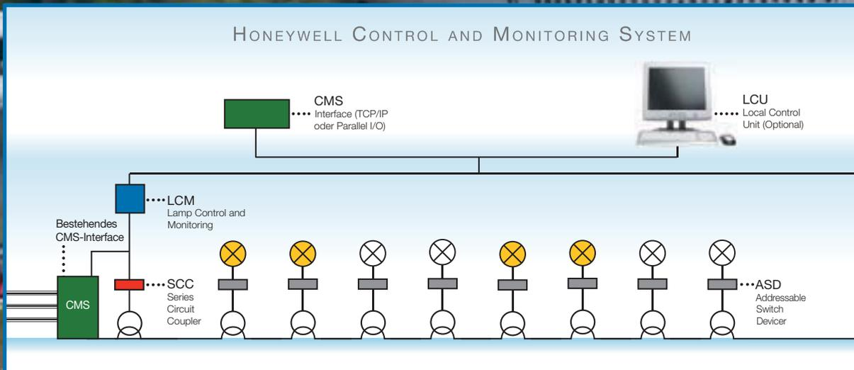
Configuring the individual lamp control system and the individual lamp control module can be carried out comfortably in the control system and is downloaded automatically, if needed. This means that the automatic configuration of each unit is backed up using the series circuit even after replacing switching modules in the field.
